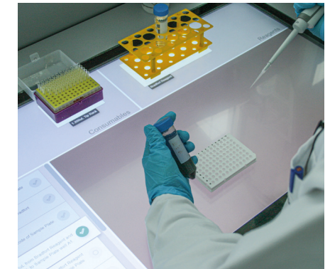
We build up a workplace for manual pipetting processes. The graphical user interface shows information about the labware at the right time and directly beside. With step-by-step instructions and a dynamic layout the laboratory staff is guided through the entire process. The workstation can be connected with other devices and software and can share information about the process, deviations in every process step, measurements like pipetted volumes and much more.
