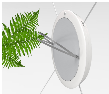
Figure 6 Design Study of a Green Wall Robot concept as a cable robot
