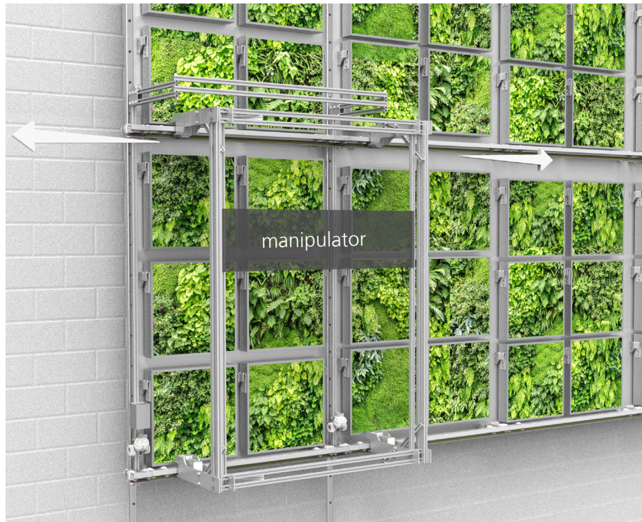
Figure 4 Visualization of a rail driven Green Wall Robot concept
